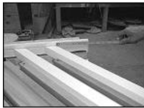
Determine center point and adjust top insert and bottom rail in jig.
