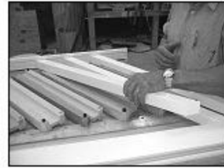
Place top insert and bottom rail on jig and adjust. Place balusters.
