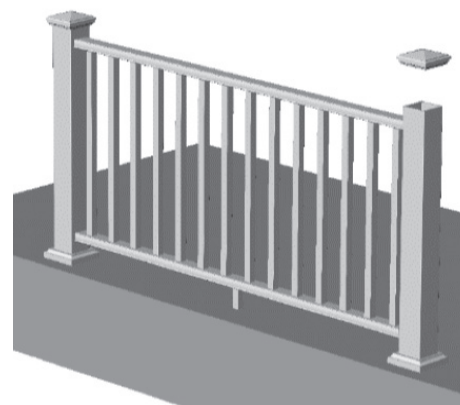
Drawing 5: Install pyramid newel caps
