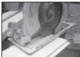
9. Optional Skill saw can be used to cut Perma Ceiling to desired width.
