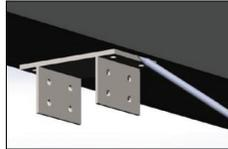
**Orientation of double-tee mounting bracket when column shaft is centered under beam.**
