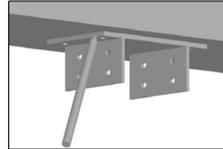
**Orientation of double-tee mounting bracket when front face of column shaft is aligned with face of foundation.**
