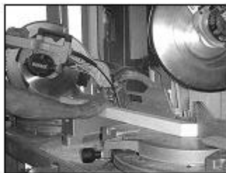
Pre-cut baluster to desired length and desired angle.
