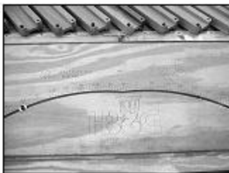
Set degree of rake. Push right for 1 1/2" baluster and push left for 1 1/4" balusters
