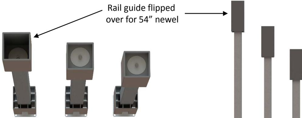
7. If not in place already, insert the top rail guide into position over the bolt extending out the top of the post mount. **Note: If you are using a 54" newel sleeve, the top rail guide of a 42" Newel-Loc™ post mount can be flipped over to accommodate the taller 54" newel.**
