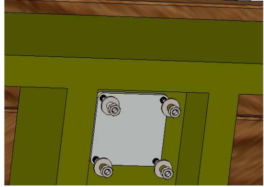
5. Under the deck, take the bottom plate, and line up the 4 corner holes in the plate with the ends of the bolts extending through the deck. Slide the bottom plate over the bolts, add the washers and nuts, and tighten the nuts securely.
